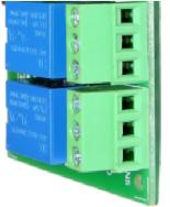
\_\_\_\_ NC - Normally closed contact - connected with common when relay is off. Disconnected while on.
